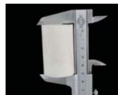
Carefully level the ring so that the top and bottom are perpendicular to the sides of the ring.
